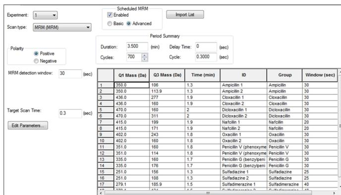
**Figure 1.** Method editor in Analyst<sup>®</sup> software version 1.6.2 used to setup the *Scheduled MRM™* Pro experiment
