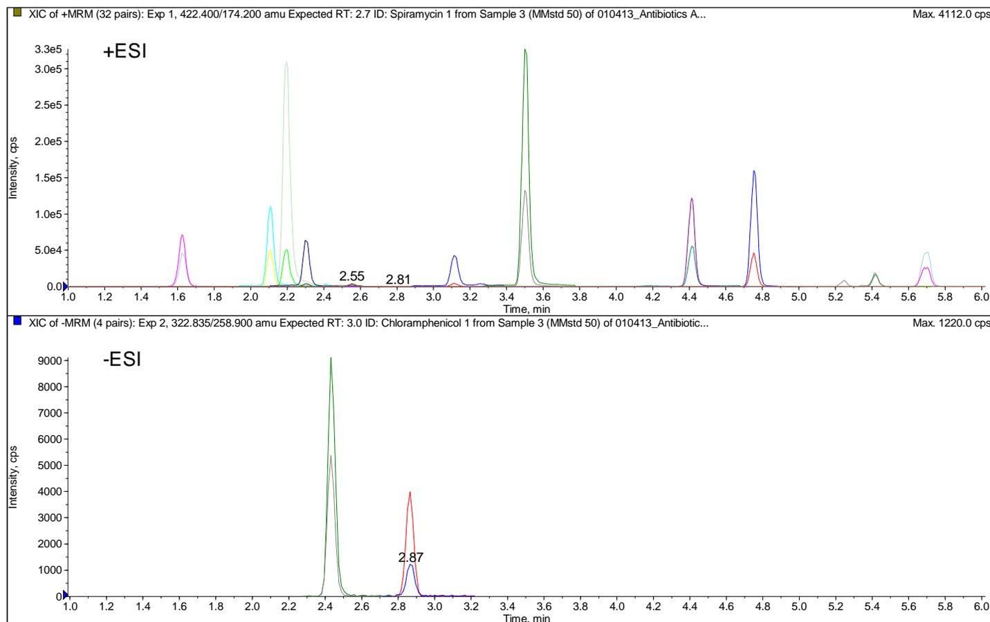
**Figure 1.** Detection of antibiotics and insecticides in a single run by LC-MS/MS using *Scheduled MRM™* with polarity switching. Positive mode (+ESI) MRM transitions shown in top pane, and XIC of all negative mode (-ESI) MRM transitions shown at bottom. Peaks are identified by retention time in Table 2.
