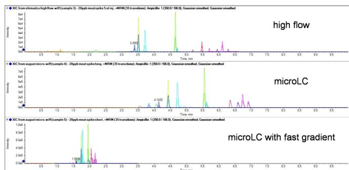
**Figure 3.** Comparison of meat sample spiked at 20  $\mu\text{g}/\text{kg}$  and analyzed by traditional high flow LC and micro flow LC-MS/MS. In this example analysis time was decreased from 10 min to 3.5 min using micro flow LC and by speeding up the gradient. In all methods peak widths at the base were 3 seconds or less.
