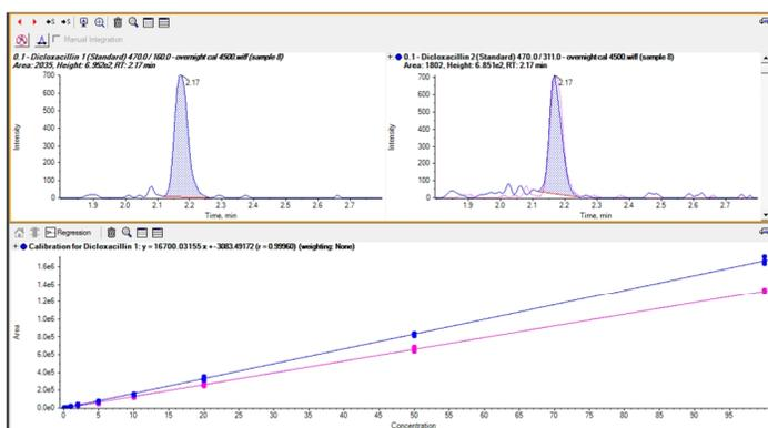
**Figure 4c.** Quantifier, qualifier MRM transition at 0.1 ng/mL (top), and calibration line of dicloxacillin from 0.1 to 100 ng/mL (bottom), the linearity is provided without the use of any internal standards
