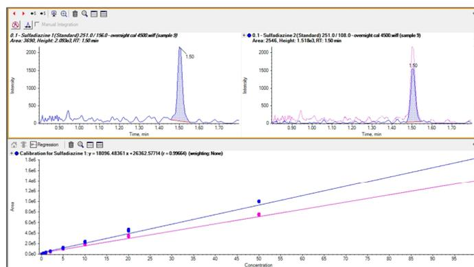
**Figure 4a.** Quantifier, qualifier MRM transition at 0.1 ng/mL (top), and calibration line of sulfadiazine from 0.1 to 100 ng/mL (bottom), the linearity is provided without the use of any internal standards
