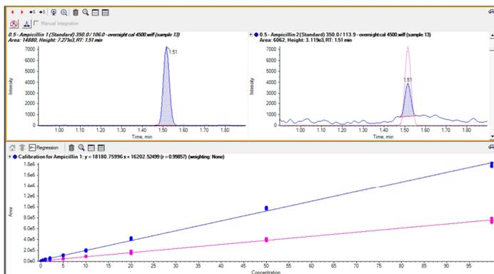
**Figure 4b.** Quantifier, qualifier MRM transition at 0.5 ng/mL (top), and calibration line of ampicillin from 0.1 to 100 ng/mL (bottom), the linearity is provided without the use of any internal standards
